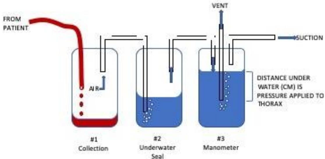
Bottle # 1 is the collection bottle for liquids, air is moved to Bottle #2, where it bubbles out underwater, preventing any air from going backwards back into the chest in the event of the suction being turned off. Bottle #3 is the manometer, or adjustment for the system. Typical wall suction is set at 160mmHg, which would be far too high a pressure and very uncomfortable for the patient. The vent is used to reduce the negative pressure, typically between 5 and 10 cmH<sub>2</sub>O.
